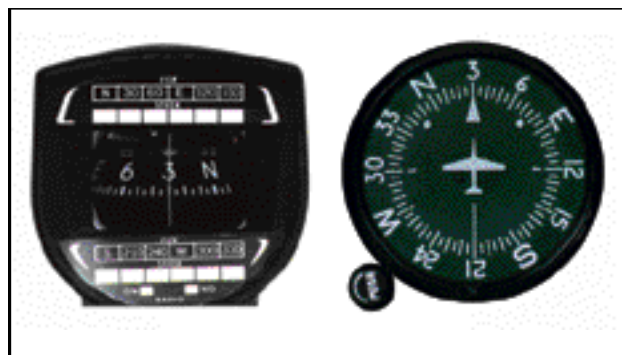
Figure 4-26. Setting the heading indicator.
